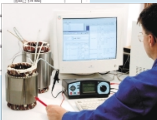
Diagnostic test of motor windings
